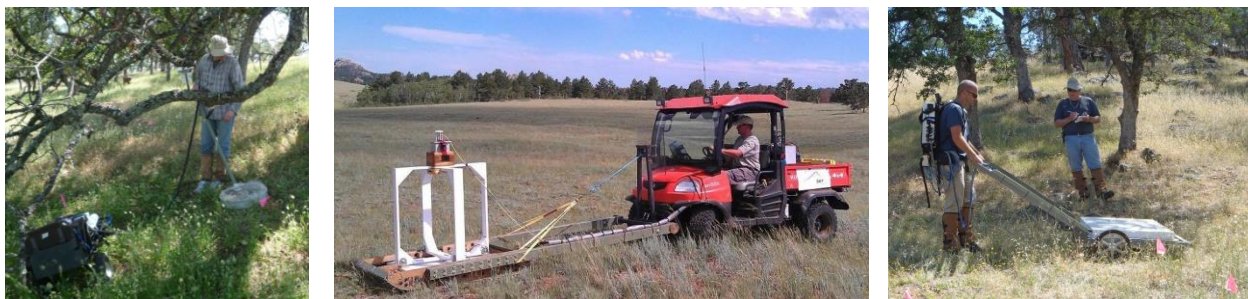
Figure 4. Advanced EMI sensors include hand-held (left), sled-mounted (middle), and cart-mounted (right) units.
