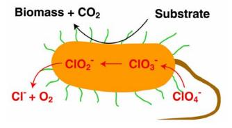
Figure 6-2. Schematic of biological reduction of perchlorate.
