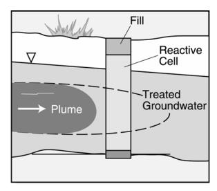
Figure 6-6. General schematic of a biobarrier.
