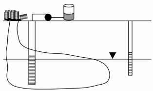
Figure 6-7. Schematic of passive in situ bioremediation.
