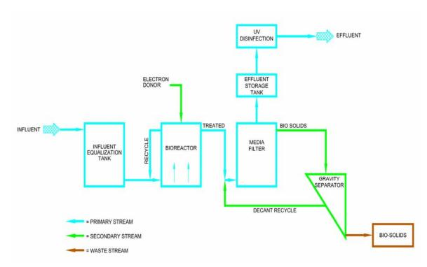
Figure 6-3. General schematic of ex situ bioremediation.
