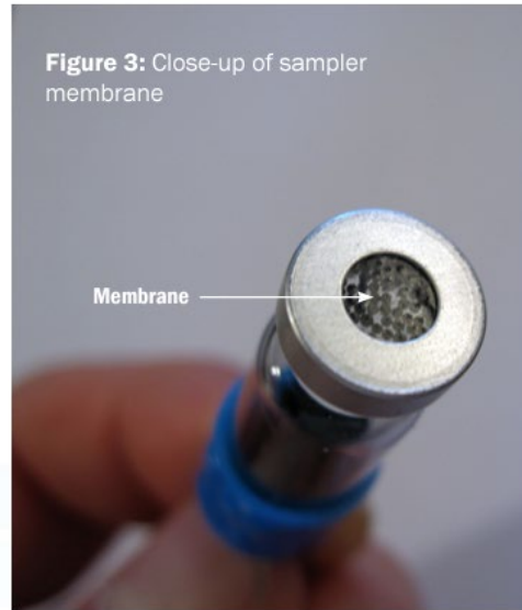
Figure 3: Close-up of sampler membrane Do not store/use WMS™ samplers near volatile chemical sources including perfume, felt markers, etc. and avoid touching the WMS™ sampler membrane (Fig 3).
