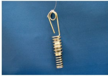
Figure 7: Deployed WMS™ sampler with line
