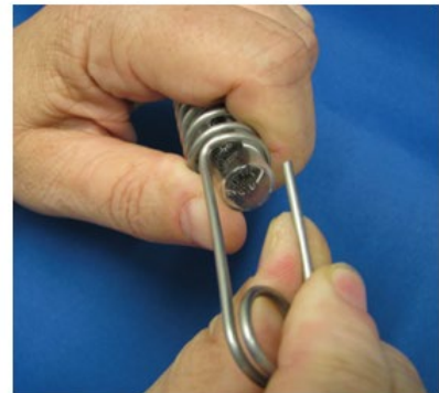
Figure 6: Bending wire to insert WMS™ sampler
