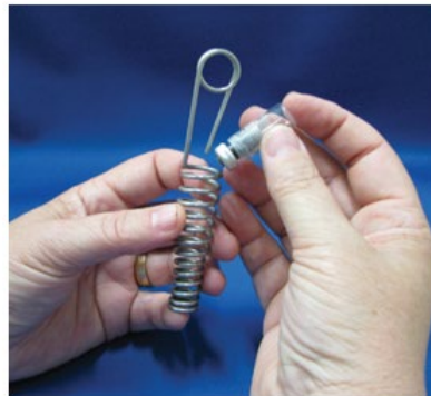
Figure 5: Aligning WMS™ sampler in wire hanger
