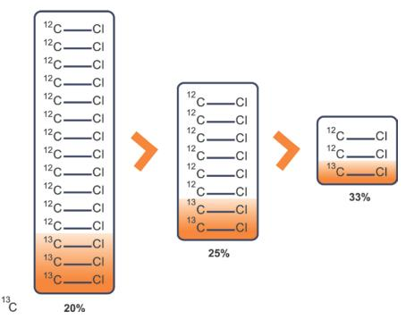
Figure 2. Illustration of <sup>13</sup>C enrichment during degradation of a contaminant with a C-Cl bond. *Source:* Microseeps, Inc., 2010, used with permission.
