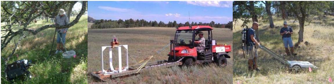
Figure 4. Advanced EMI sensors include hand-held (left), sled-mounted (middle), and cart-mounted (right) units.
